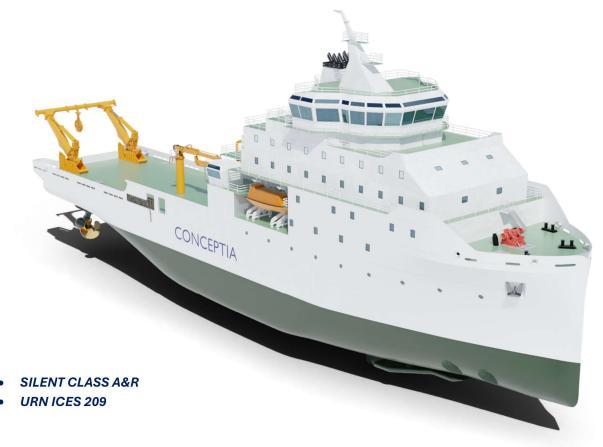
Conceptia is engaged in the basic and detailed design of an advanced research ship tailored for sophisticated acoustic research. This vessel features a state-of-the-art diesel-electric propulsion system, ensuring efficient and reliable operation. Additionally, it is equipped with dynamic positioning capabilities for precise maneuvering during data collection
